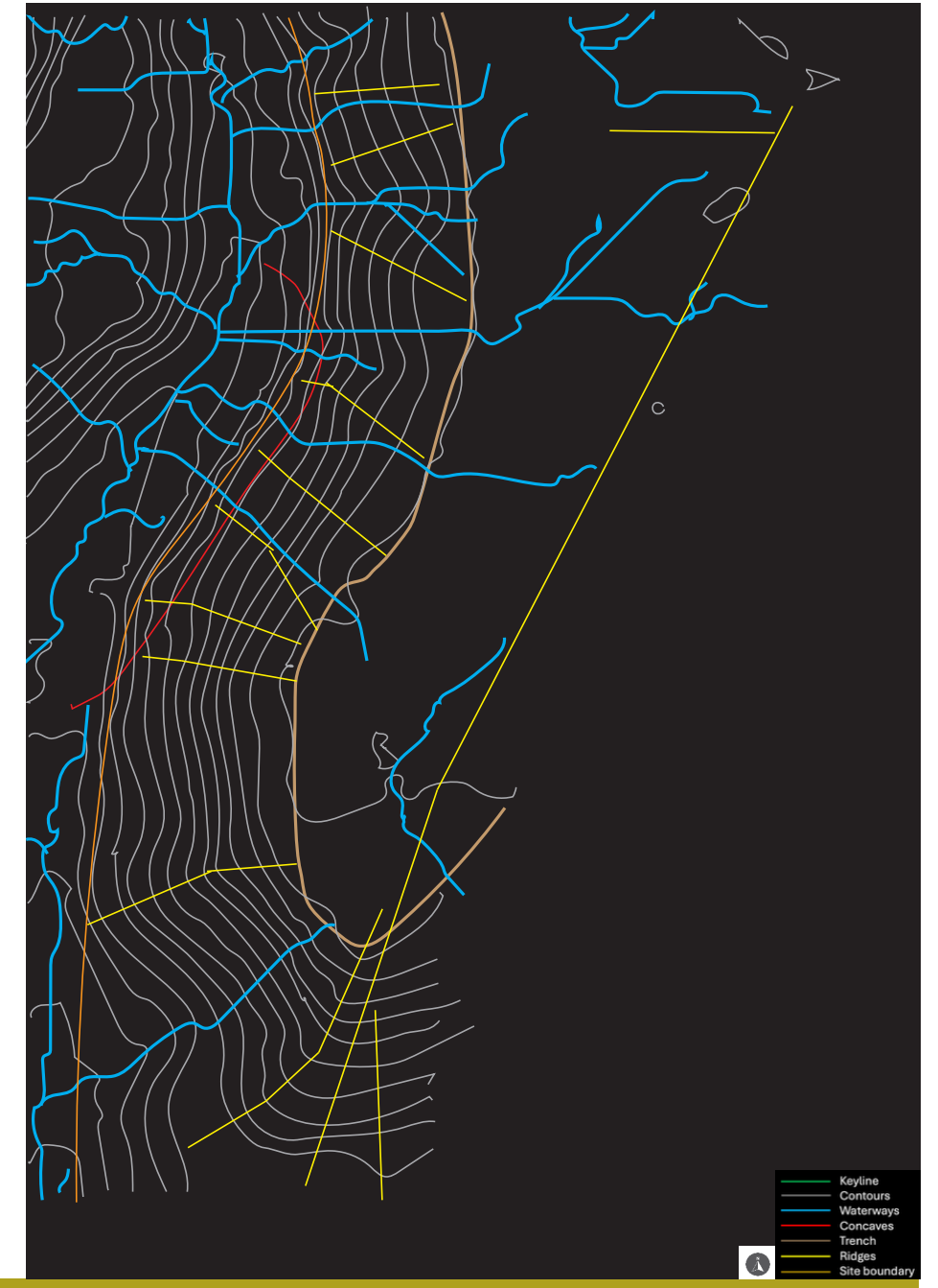
Figure 34. Western slope next to the boulevard Lazaro Cardenas, showing contours, waterways in valleys, ridges, and concave areas with potential landslides in red [Source: by the authors].
